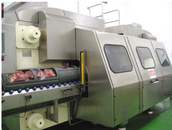
Fig. 7.2 NC Hyperbaric industrial equipment for HPP up to 650 MPa located at IRTA-CENTA (Monells). About 120 L capacity, 300 mm inner diameter
